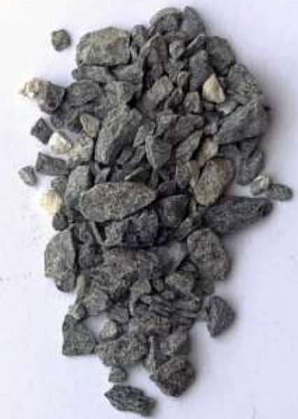
Aggregate 3/16 = 05 MM - 10 MM
