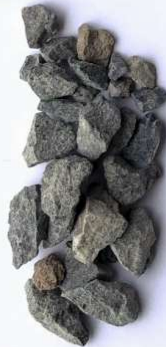
Aggregate 3/8 = 10 MM - 20 MM
