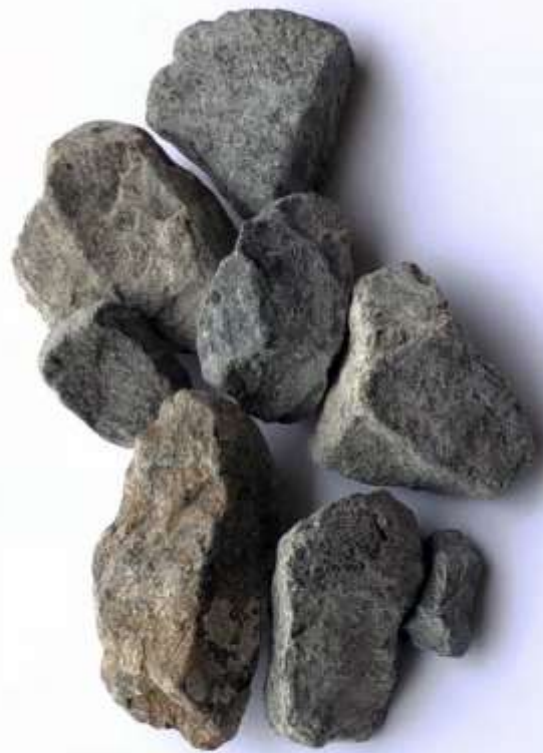
Aggregate 3/4 = 20 MM - 30 MM
