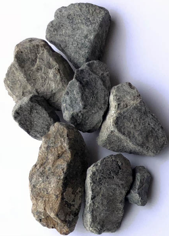
Aggregate 3/4 = 20 MM - 30 MM
