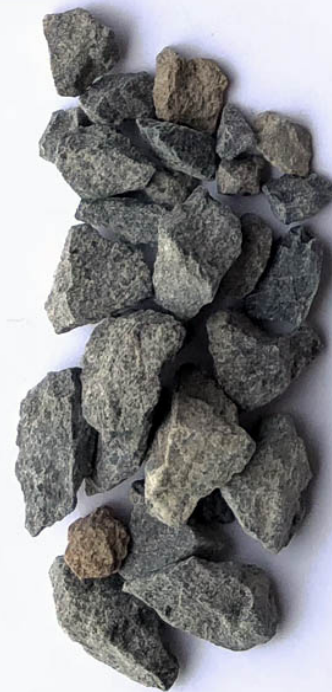
Aggregate 3/8 = 10 MM - 20 MM
