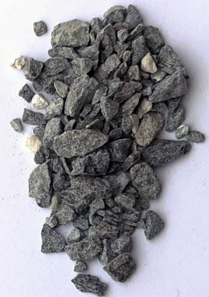
Aggregate 3/16 = 05 MM - 10 MM
